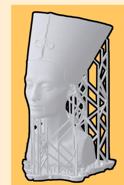
**Formlabs support** is made of a **scaffolding-like structure**, which reaches up to all the parts of the print. This support has to be cut off using snips, available in the workshop.
